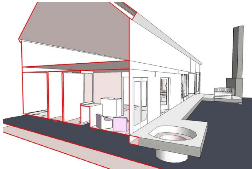
Section throught Spa Room (Bathroom)
